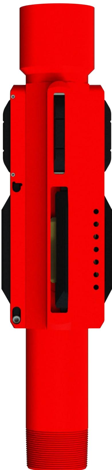
The **Centralized Advanced Torque Anchor (CATA)** is a simple and reliable solution for preventing tubing back-off in PCP pump applications. Equipped with drag blocks, it anchors the PCP in horizontal wells while keeping the system centralized. Its wedge-shaped anchoring blocks bite into the casing wall when right-hand torque is generated in the tubing string. These blocks are spring-loaded, ensuring immediate torque transfer to the casing.
