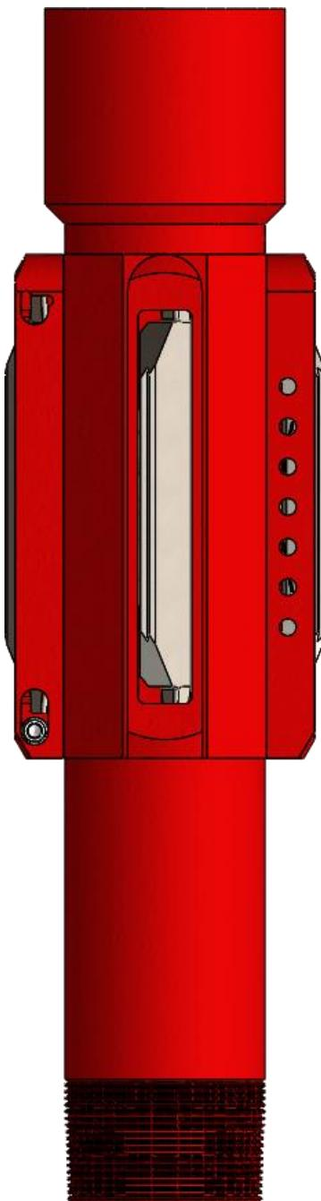
The **Evolution Advanced Torque Anchor (ATA)** is designed to transfer the PC Pump torque to the casing walls. The ATA uses wedge shaped anchoring blocks to bite into the casing wall when right hand torque is generated in the tubing string. These anchoring blocks are spring loaded so the transfer of torque to the casing is immediate. Its best applications are in deep wells, horizontal wells or heavy oil situations.
